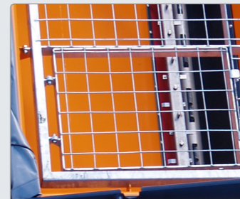
The safety grate features an inspection door for quick access to the hopper.
